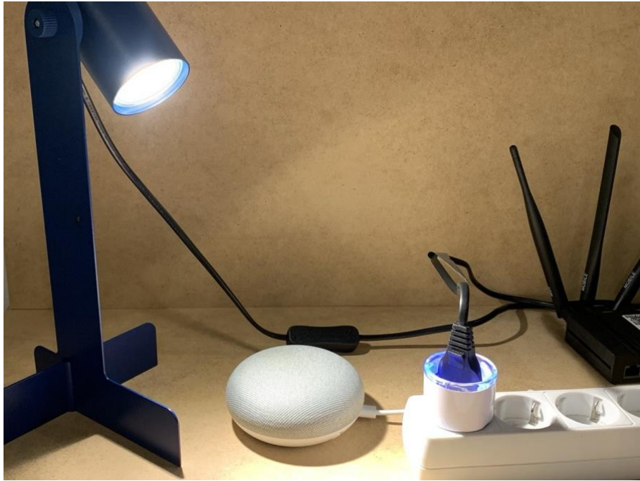
Figure 13 — lamp connected to a smart outlet and Google Nest Mini smart speaker
